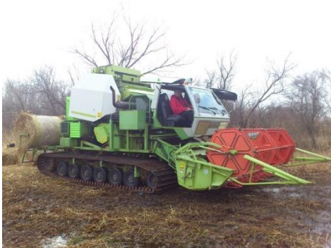
Figure 5. Harvester for fully grown reed “Sumo-Quaxi”, during the harvesting operation Source: own photo.
