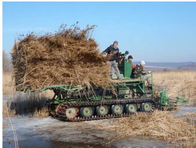
Figure 4. Harvester for young grown reed “Paul 1”; harvesting on ice Source: own photo.
